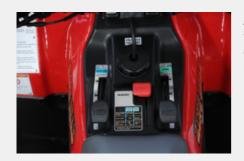
Abundant low-mid range torque and the unique versatility of a 3-speed sub-transmission with high, low and super-low ranges means there's a gear for every situation. The three drive modes – 2WD, 4WD and front diff-locked 4WD – are all easily accessed via control levers just forward of the seat.
