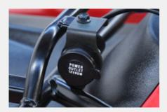
High-capacity generator. The 12-volt DC outlet is ideal for using various electric accessories.
