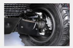
Front disc brakes with twin piston calipers for strong stopping power, wet or dry.
